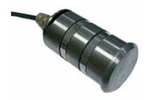
${\it Tensiometer pins are usually used for winches.}$
