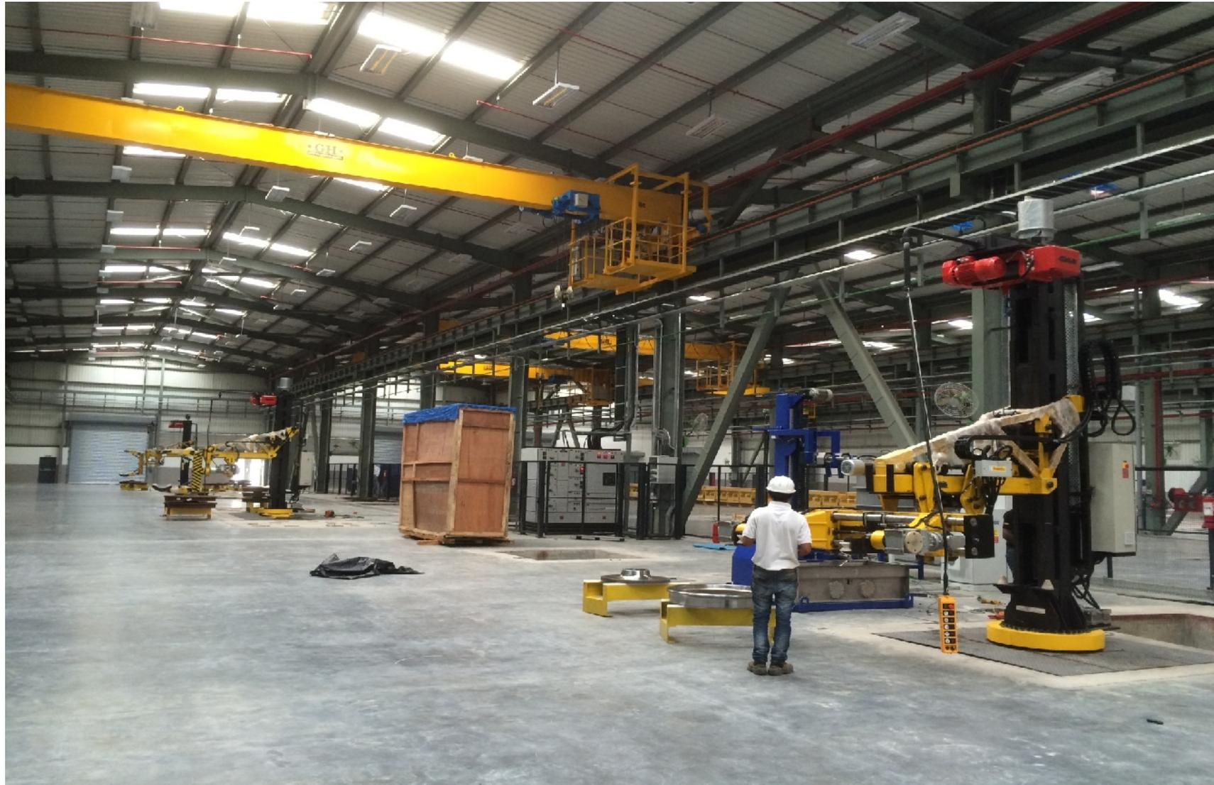
1. Engine Valve Handling & Inspection by Robot
